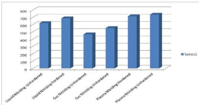
**Fig 3.7** Nitriding Process Vs Obtained Hardness
