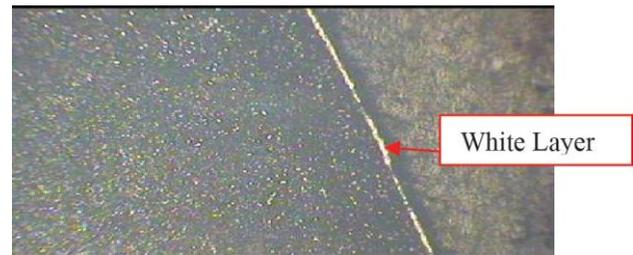
**Fig 3.2** Liquid Nitrided- EN 19 @ 100X without Hardened & Tempered Conditions.
