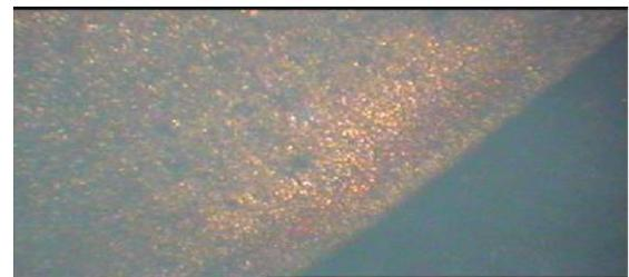
**Fig 3.4** Gas Nitrided - EN 19 @ 100X without Hardened & Tempered Conditions.
