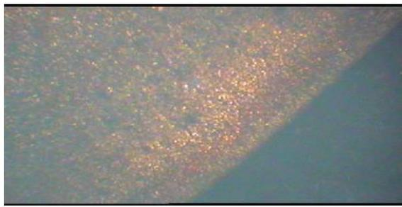
**Fig 3.6** Plasma (Ion) Nitrided - EN 19 @ 100X without Hardened & Tempered Cond.
