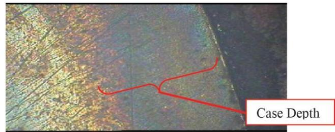
**Fig 3.1** Liquid Nitrided- EN 19 @ 100X with Hardened & Tempered Conditions.
